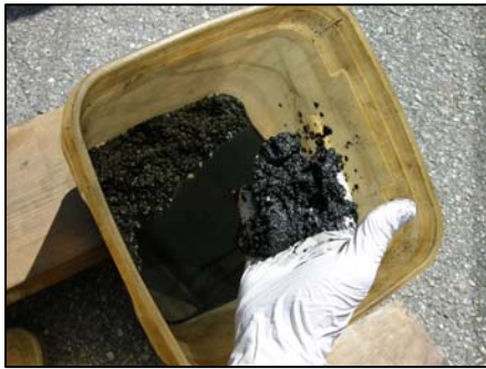
Debris and water removed from the bottom of the fuel/water separator.
